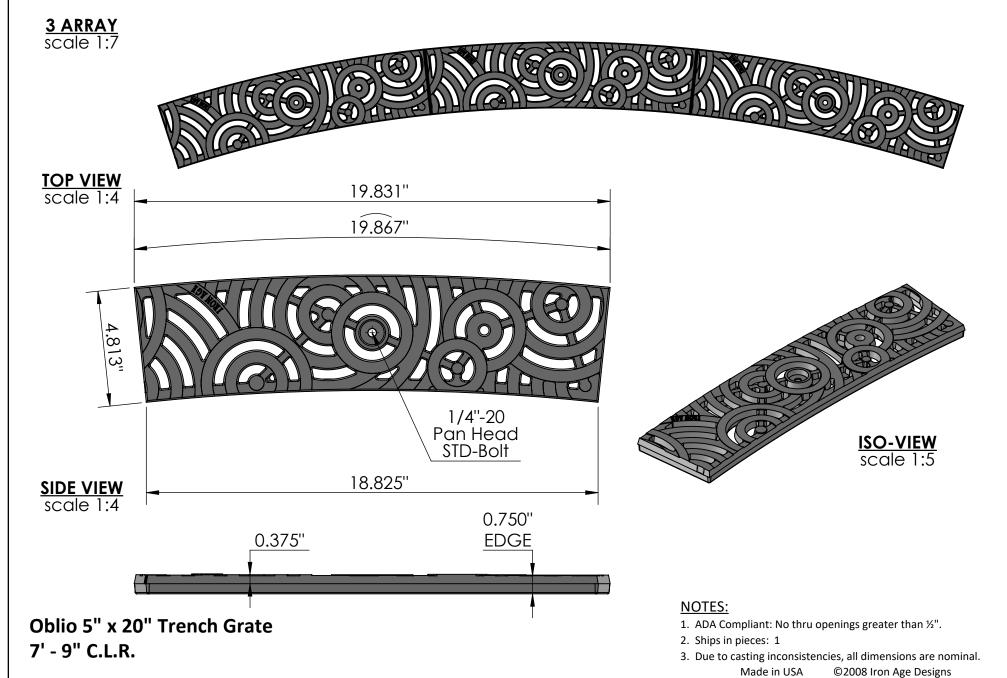
Material: Ductile Iron 65-45-12 Weight: 10.00 lbs. Free Drain Area: 20.75 in/sq., or 22.27 By: MS Checked: MS **Date:** 4-26-22 .060 CuFt./sec. © Registration: Raw Edge: 0.750" Flow Rate: GPM, or Scale: NTS 27.18 Pending DESIGNS Iron Age Custom Frames **Product ID:** 206.276.0925 Fits: Drawing Name: 02 OBL I 5x7'-9"CLR TrenchGrate **SOLD SEPARATELY** OR5-201998 Page 1 www.ironagegrates.com
