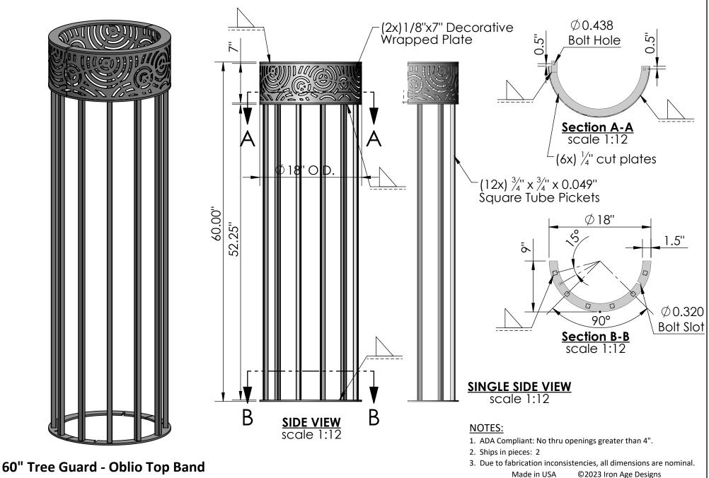
Material: Mild Steel By: JH Checked: JH **Date**: 10-12-23 Finish: Powdercoat - BK59 Black Texture © Registration: Scale: NTS Pending
